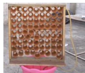
Gambar 6. Panel honeycomb air cooler
