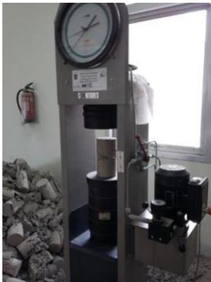
**Gambar 7.** *Universal Testing Machine* (UTM)
